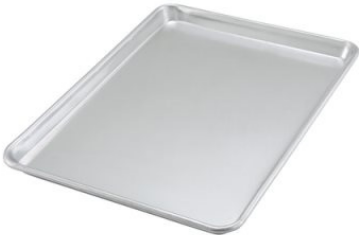
Sheet Pan/Serving Tray, 1/2 size, 13" x 18", closed bead, 20 gauge, 3003 aluminum.
